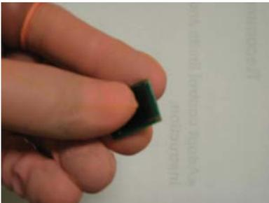
**Fig. 4** Avoid this method of display handling
