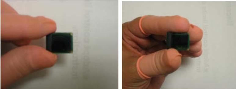
**Fig. 3** Best method of handling the displays
