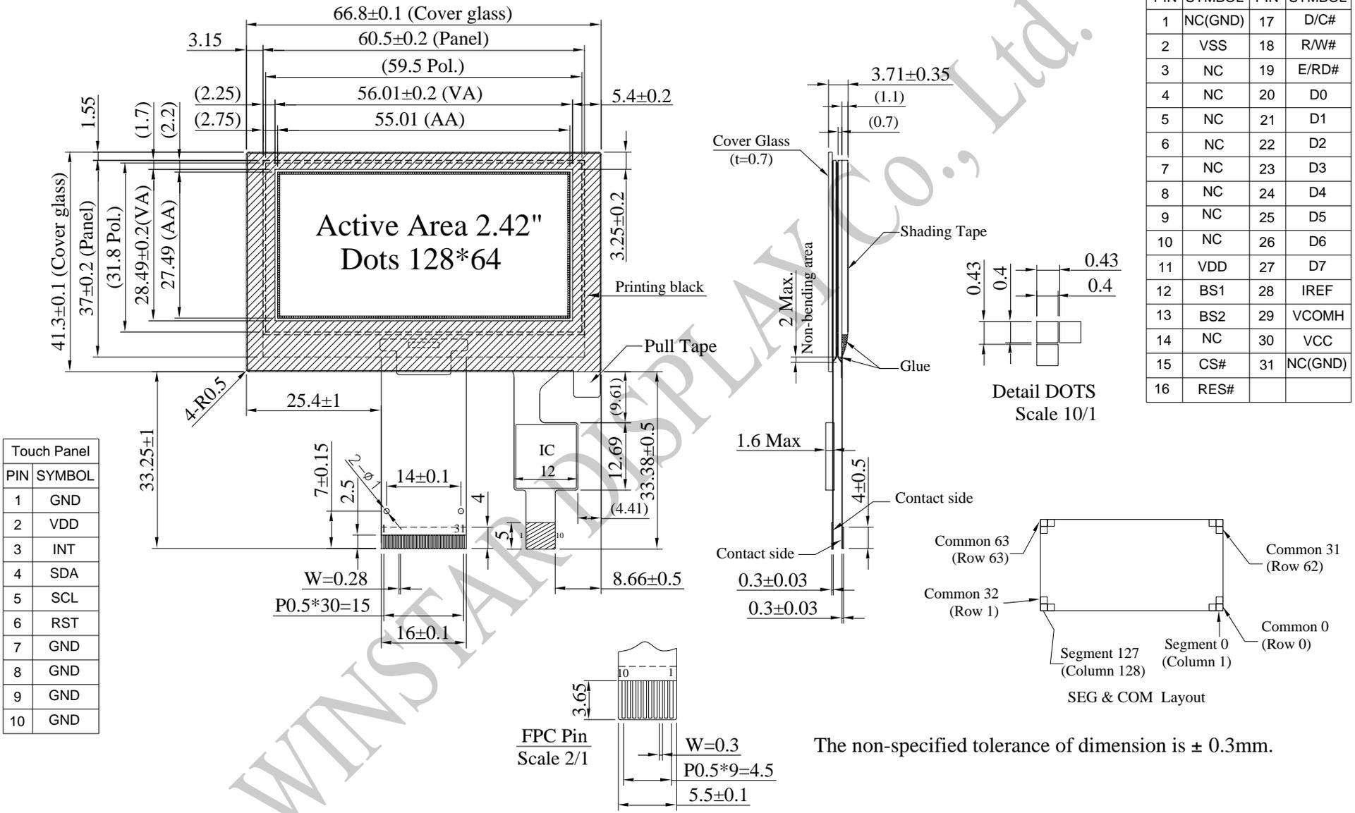
The non-specified tolerance of dimension is ± 0.3mm.
