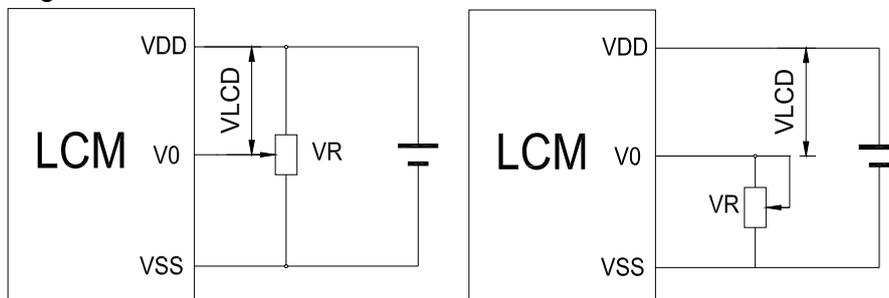
V<sub>DD</sub>-V<sub>0</sub>: LCD Driving voltage
