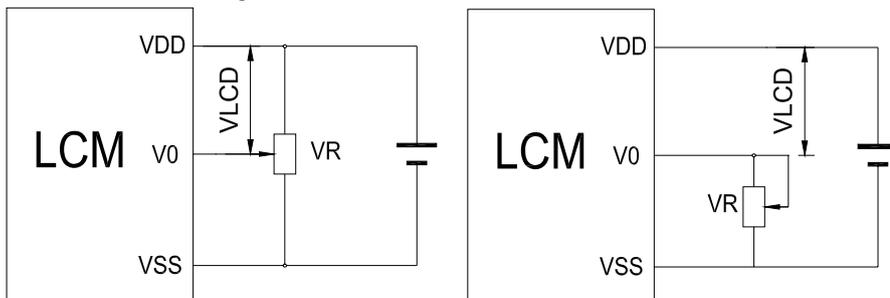
V<sub>DD</sub>-V<sub>0</sub>: LCD Driving voltage
