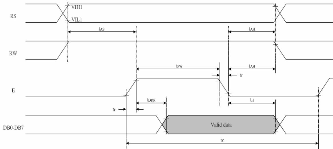
**Write cycle** (Ta=25°C, VDD=5.0V)
