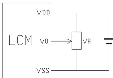
V<sub>DD</sub>-V<sub>0</sub>: LCD Driving voltage
