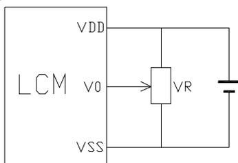
V<sub>DD</sub>-V<sub>0</sub>: LCD Driving voltage
