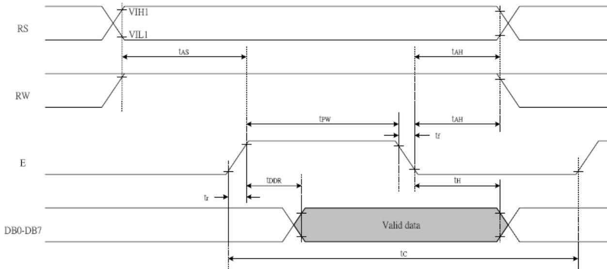
**Write cycle (Ta=25°C, VDD=5.0V)**
