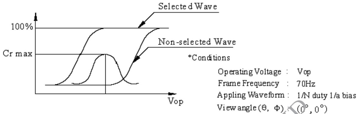
$$\text{Contrast ratio}(Cr) = \frac{\text{Brightness of selected dots}}{\text{Brightness of non-selected dots}}$$
