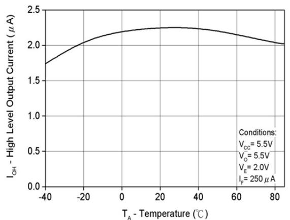
**Fig 6 High Level Output Current vs T<sub>A</sub>**
