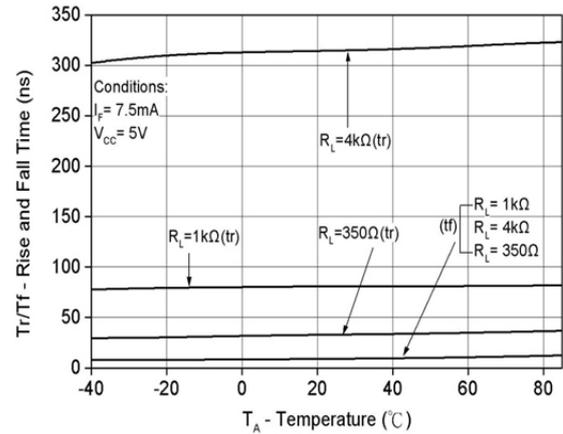
**Fig 10 Rise and Fall Time vs  $T_A$**
