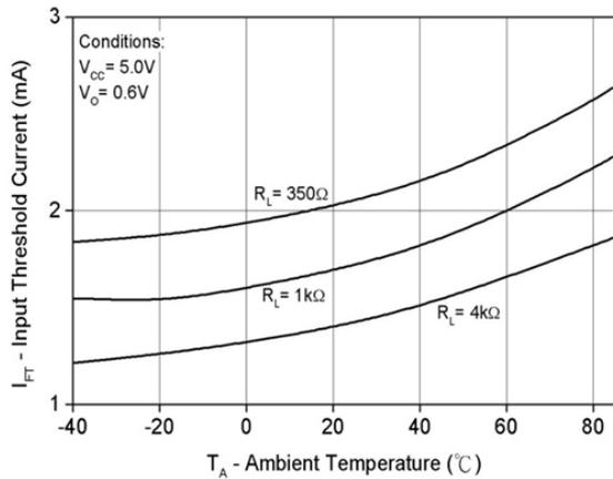
**Fig 3 Input Threshold Current vs T<sub>A</sub>**
