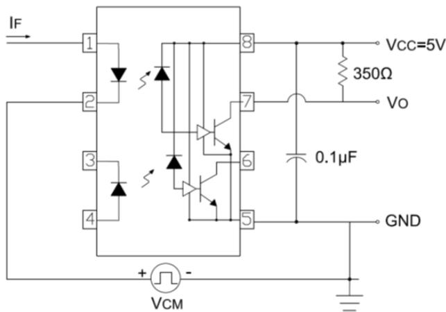
**Fig 12 Common Mode Transient Immunity Test Circuit**
