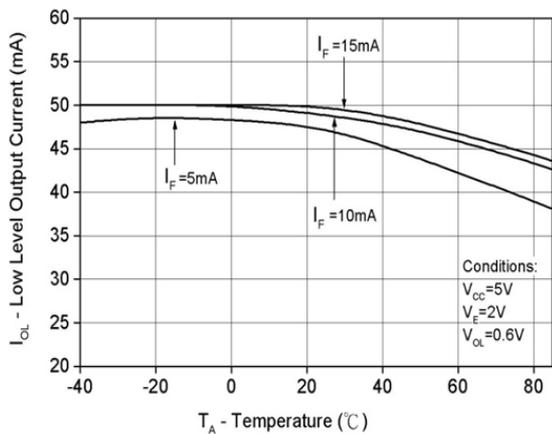
**Fig 5 Low Level Output Current vs T<sub>A</sub>**
