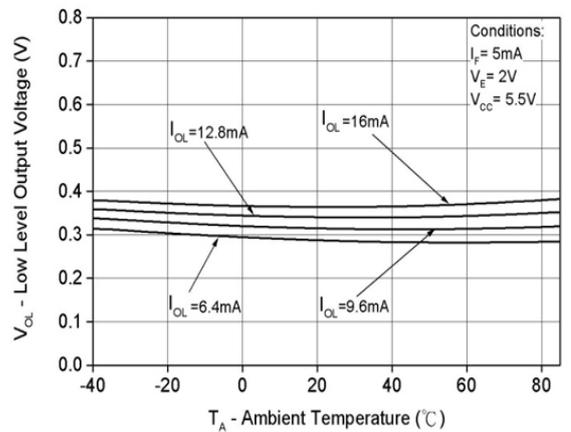
**Fig 4 Low Level Output Voltage vs T<sub>A</sub>**
