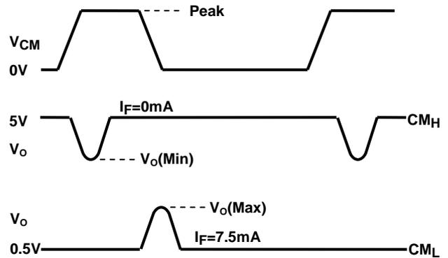
Common mode transient immunity in logic high level is the maximum tolerable (positive)  $dV_{CM}/dt$  on the leading edge of the common mode pulse signal  $V_{CM}$ , to assure that the output will remain in a logic high state (i.e.,  $V_o > 2.0V$ ).
