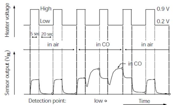
Fig 2 SB-500-12: Operating conditions and output signal
