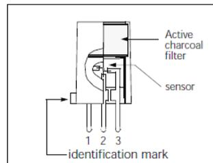
Fig 1c. Pin Layout
