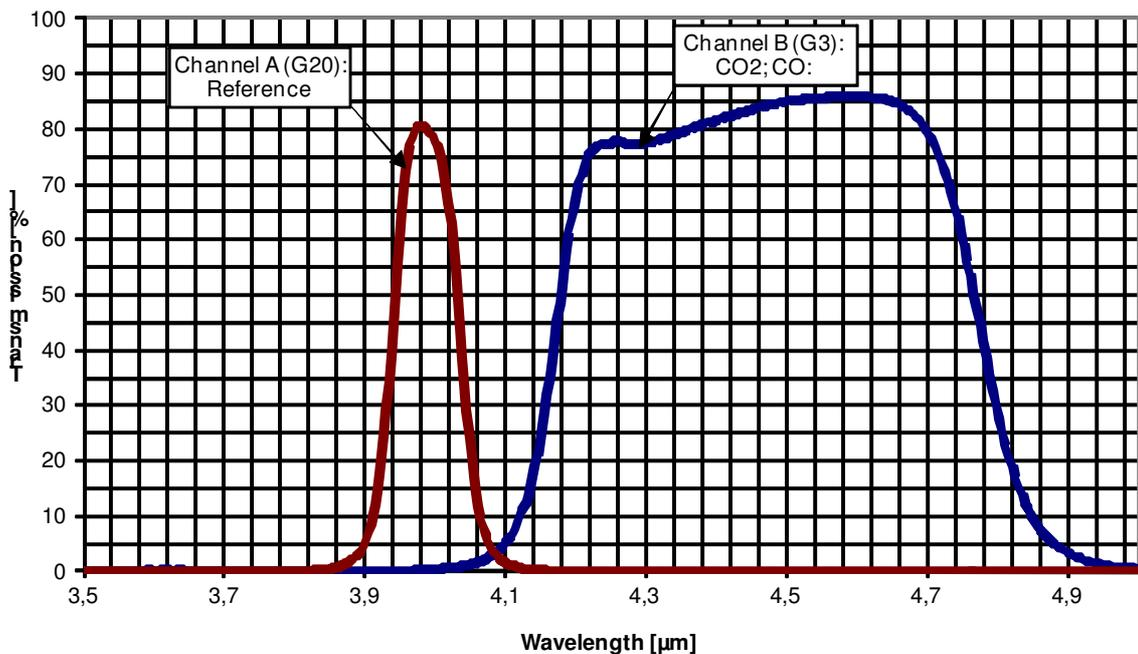
Fig. 4: Filter Transmission
