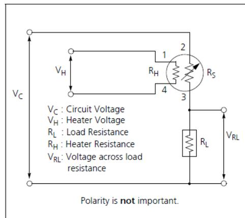
Fig 2. Standard circuit
