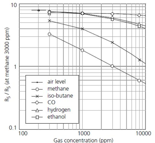
Fig 3. Sensitivity characteristics
