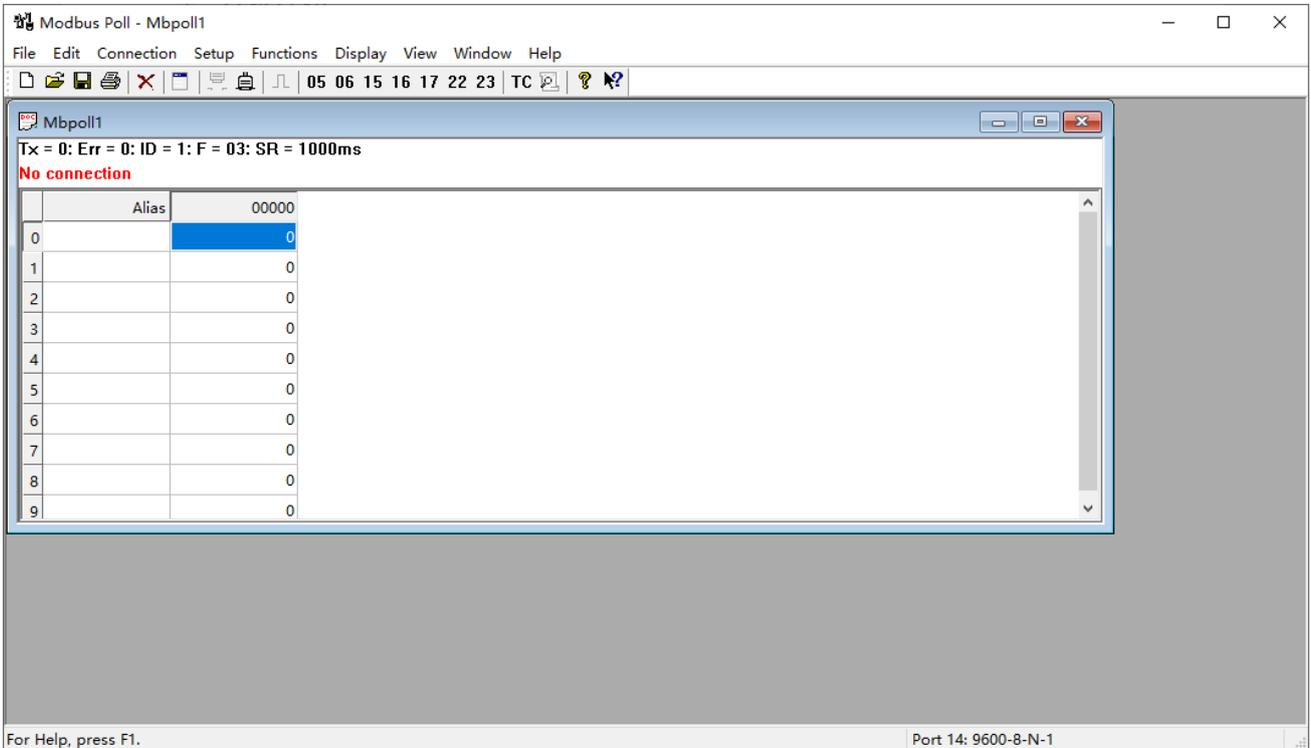
Configure connection parameters: Baud rate 9600bps, one start bit, 8 data bits, no verification, one stop bit.
