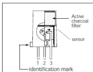
Fig 1c. Pin Layout
