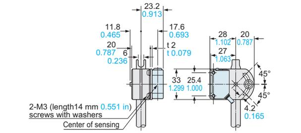
**Assembly dimensions with RF-210 (Reflector) (Mounting part only)**
