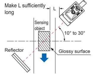
**Retroreflective type sensor with polarizing filters (CX-491□)**
