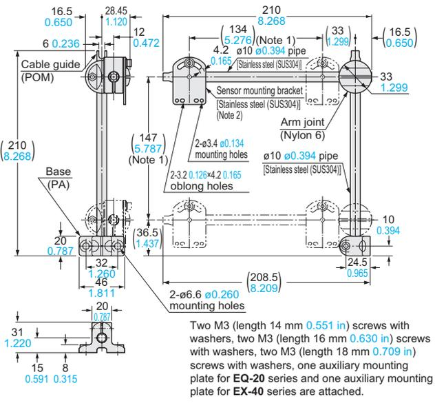
Notes: 1) The dimensions in the brackets indicate the adjustable range of the movable part.
