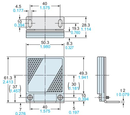
Material: Cold rolled carbon steel (SPCC)
