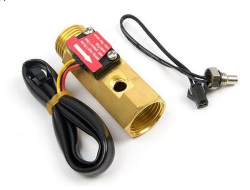
It consists of a copper body, a water rotor, and a hall-effect sensor. When water flows through the rotor, rotor rolls. Its speed changes with different rate of flow. The hall-effect sensor outputs the corresponding pulse signal.
