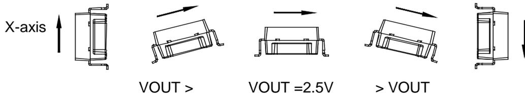
**Figure 8.** The measuring direction of the SCA61T
