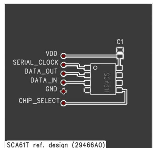
**Figure 14.** SPI connection example
