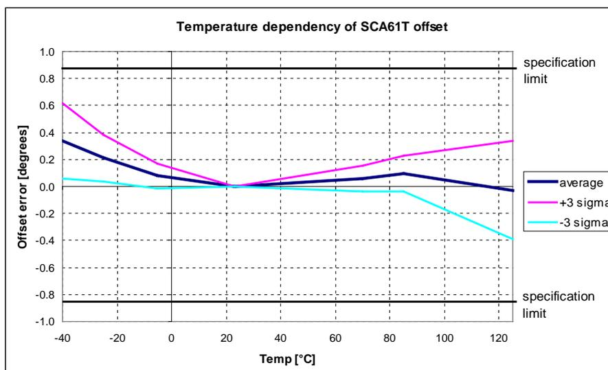
**Figure 4.** Typical temperature dependency of the SCA61T offset
