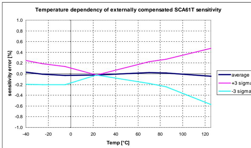
Figure 7. The temperature dependency of externally compensated SCA61T sensitivity
