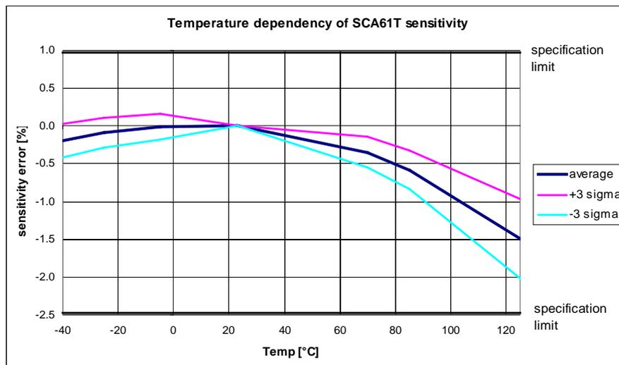
**Figure 5.** Typical temperature dependency of SCA61T sensitivity
