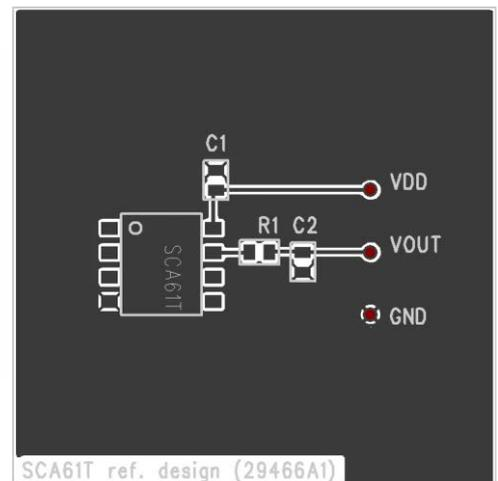
**Figure 13.** Analog connection and layout example
