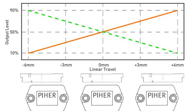
Custom output functions with up to 4 programmable points on request.
