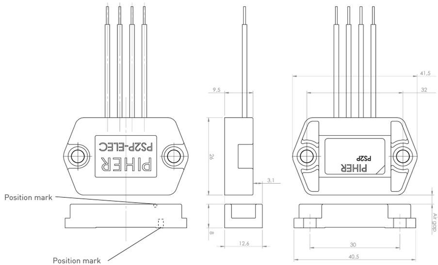
Magnet shown on 50% position. Nominal air gap: 3mm, higher on request
