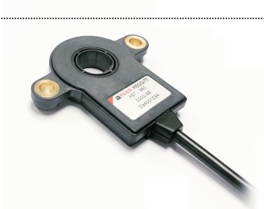
The PST-360 through / hollow shaft position sensors combines three critical design features; 1) through hole where the shaft passes through the sensor, 2) high accuracy absolute position feedback over up to 360°, and 3) a true non-contacting sensing element. Piher's design does not rely on gears or other rotating parts.
