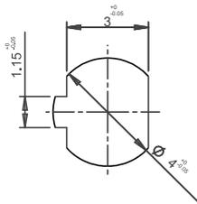
Shaft should be ferromagnetic material. If you want to use a non-ferromagnetic shaft please contact Piher.
