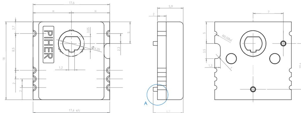
Rotor is shown at zero position. Sensor is delivered at random position
