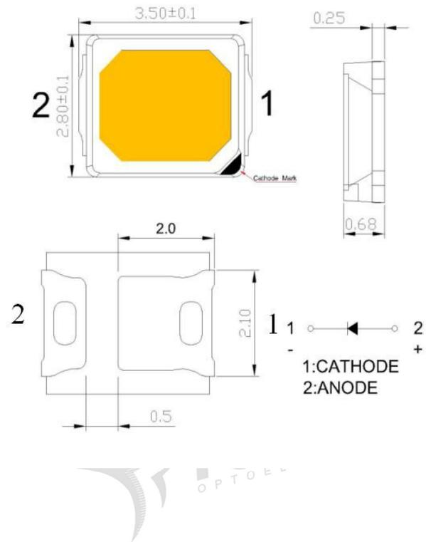
**Recommend Soldering pad design(unit=mm)**
