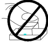
When handling the product with tweezers, LEDs should only be handled from the side and make sure that excessive force is not applied to the resin portion of the product. Failure to comply can cause the resin portion of the product to be cut, chipped, delaminated and/or deformed, and wire to be broken, and thus resulting in catastrophic failure.
