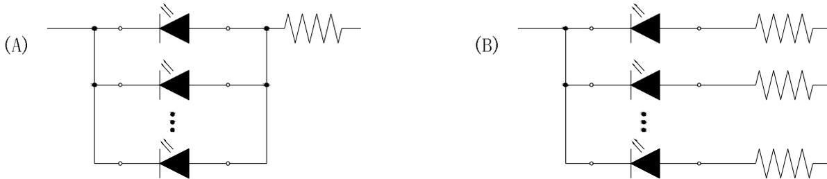
• This product should be operated in forward bias. A driving circuit must be designed so that the product is not subjected to either forward or reverse voltage while it is off. In particular, if a reverse voltage is continuously applied to the product; such operation can cause migration resulting in LED damage.
