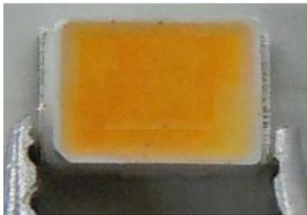
(3) When populating boards in SMT production, there are basically no restrictions regarding the form of the pick and place nozzle, except that mechanical pressure on the surface of the resin must be prevented. This is assured by choosing a pick and place nozzle which is larger than the LED's reflector area.
