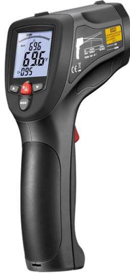
Provide much faster, easier and accurate readings for most surface temperature measurements with Dual laser pointers. Two laser points converge to a single spot when the unit is at the optimal distance from the object being measured.
