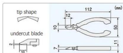
NS-06 ESD-safe. Undercut blade for work in a confined space. With angle adjuster
