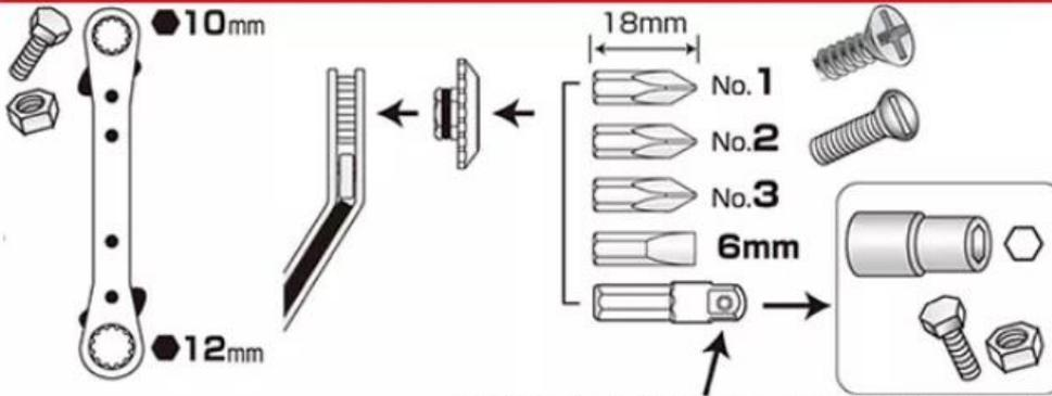
1/4" (6.35mm) socket 'adapter' accepts standard 1/2" sockets, allowing the dr-56 to be used like a ratchet socket wrench!
