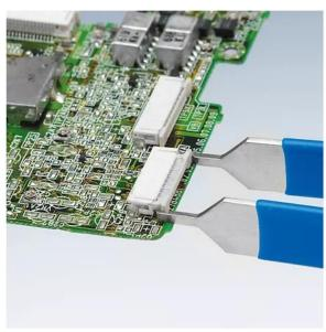
Accurately-designed tips works well to insert or extract the connector mounted at right angles on highly-dense PCB.
