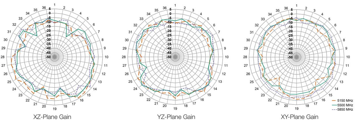
Radiation Patterns - Edge of Ground Plane Bent 90 Degrees
