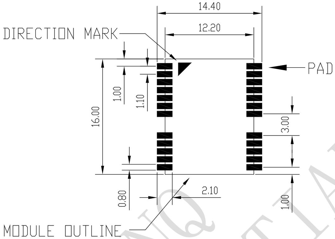
Figure 4 Recommended PCB decal (top view) (Unit: mm)
