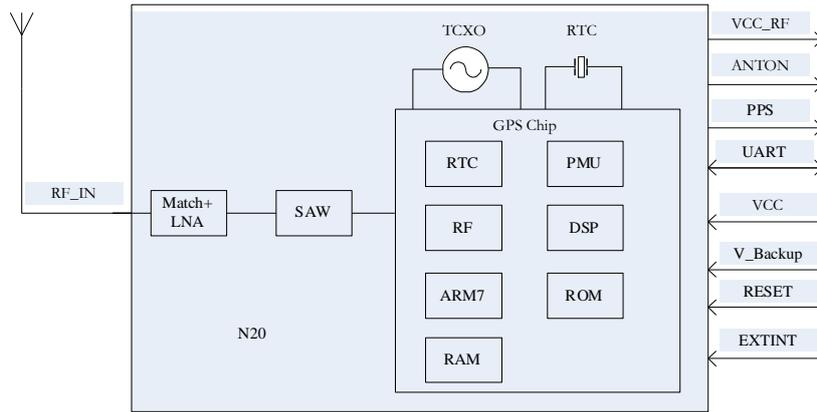
Figure 1 N20 functional diagram
