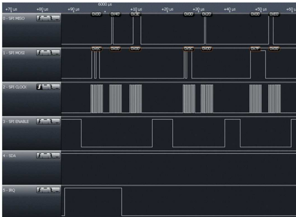
Figure 6-24. IRQ With One Byte in FIFO
