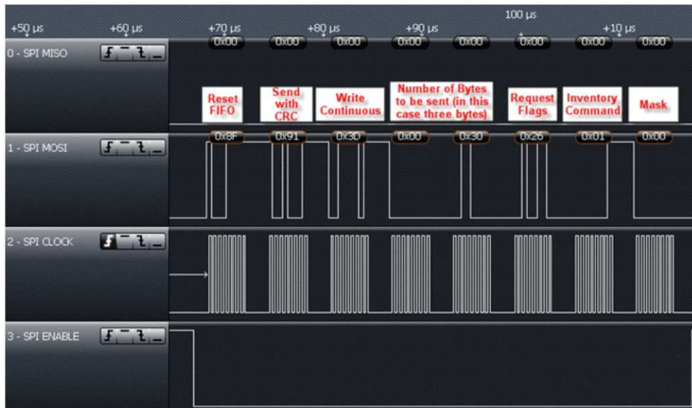
Figure 6-20. Inventory Command Sent From MCU to TRF7960A
