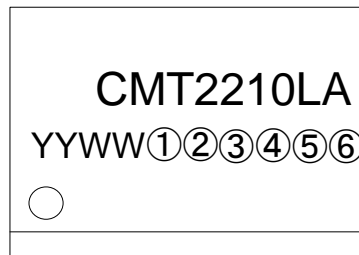
Figure 16. CMT2210LA Top Marking in SOP8 Package
