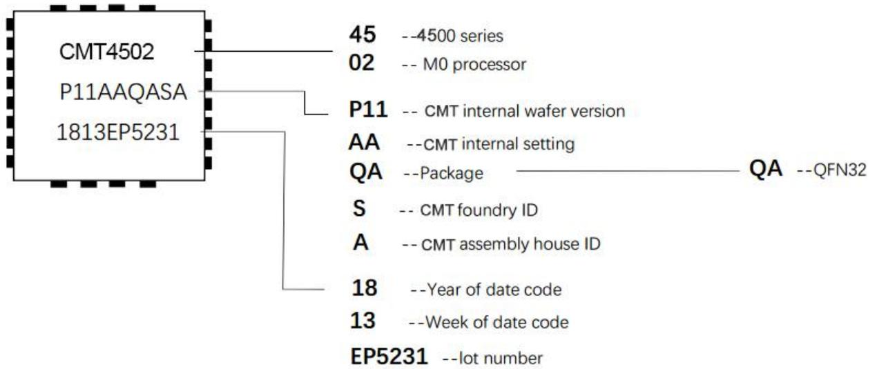
Figure 14: Chip Marking
