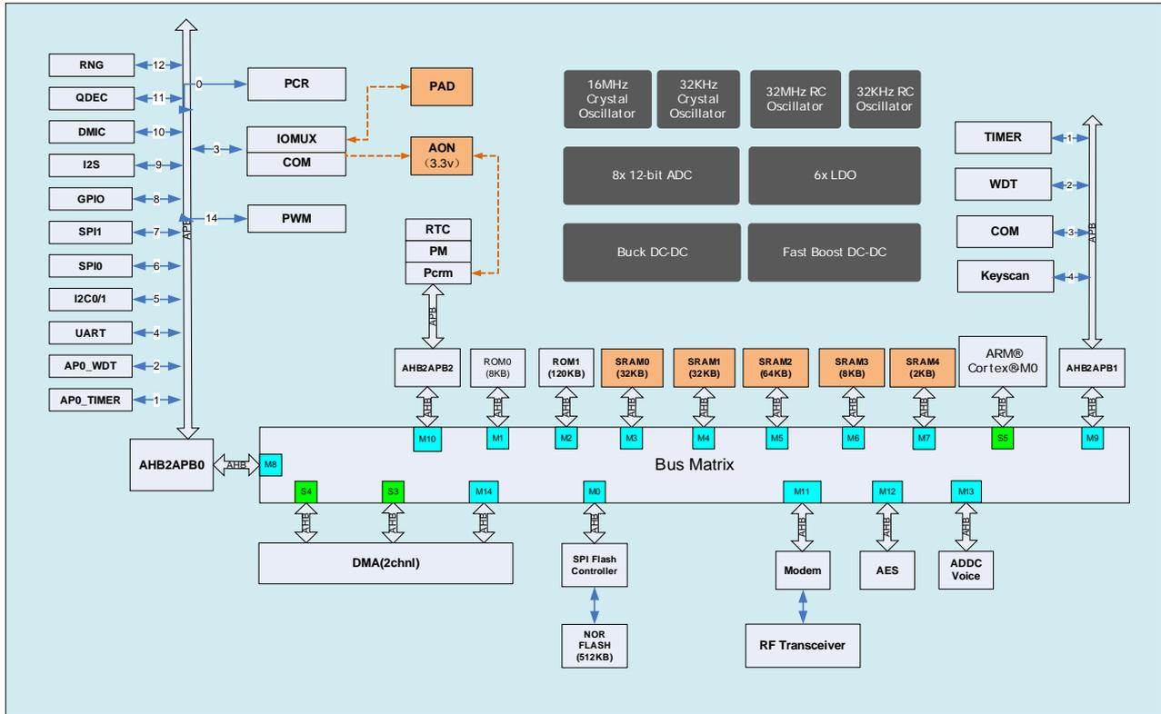
Figure 1: CMT4502 block diagram
