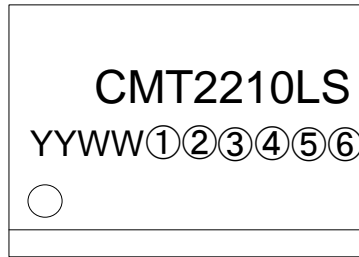
Figure 12. CMT2210LSW Top Marking
