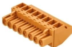
Female plugs with clamping-yoke connection for connecting wires with a right-angle (90° or 270°) outlet direction. The female connectors provide space for labelling and can be coded. Fastened by means of a flange or release latch. They also provide an integrated plus/minus screw, protection against faulty insertion of the wire, and they are delivered with open clamping yokes. HC = High Current.
