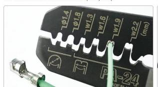
Round Dies (For DuPont contact etc.) [ $\phi$ 1.4 &  $\phi$ 1.8mm] Wrap triangular lugs of the barrel around the insulation without damage.
