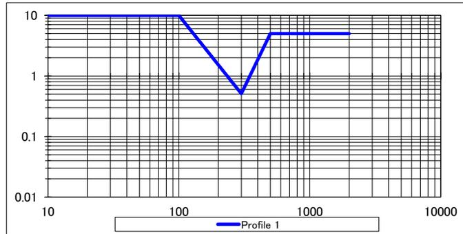
**Random Vibration Profile 2**     $-40\text{ }^{\circ}\text{C} < T < 125\text{ }^{\circ}\text{C}$
