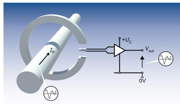
Fig. 1: Principle of the open loop transducer.
