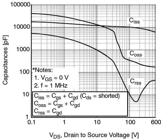
Figure 5. Capacitance Characteristics
