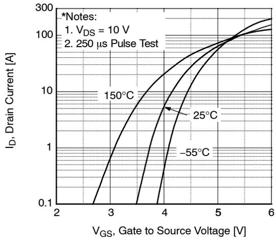
Figure 2. Transfer Characteristics
