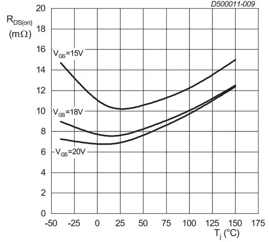
$I_{DS} = 100\text{ A}; t_p < 200\ \mu\text{s}$
