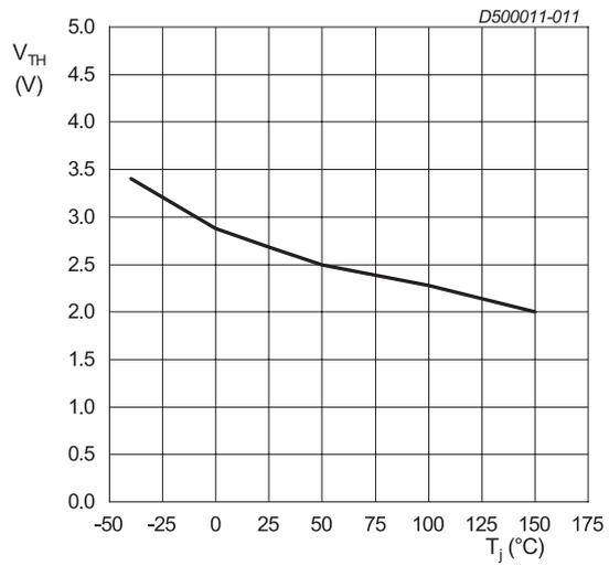
$V_{DS} = 10\text{ V}; I_{DS} = 40\text{ mA}$
