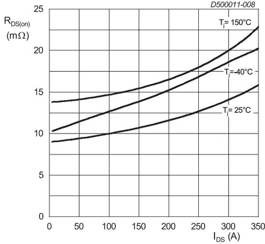
$V_{GS} = 15\text{ V}; t_p < 200\ \mu\text{s}$
