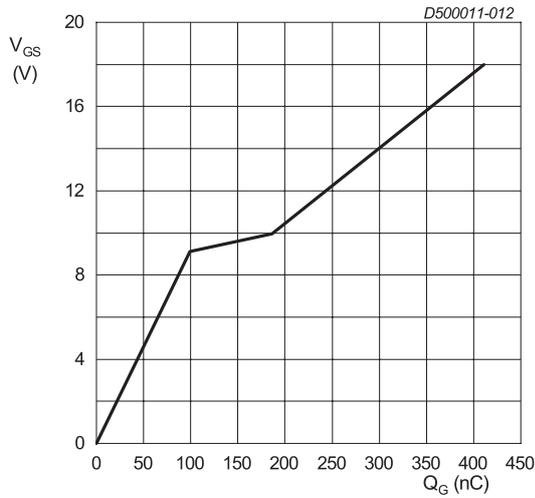
$I_{DS} = 100\text{ A}; I_{GS} = 1\text{ mA}; V_{DS} = 800\text{ V}; T_j = 25\text{ }^\circ\text{C}$
