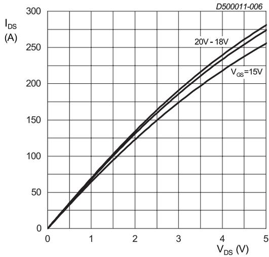
$T_j = 150\text{ °C}; t_p < 200\ \mu\text{s}$
