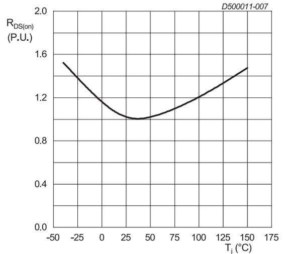
$I_{DS} = 100\text{ A}; V_{GS} = 15\text{ V}; t_p < 200\ \mu\text{s}$
