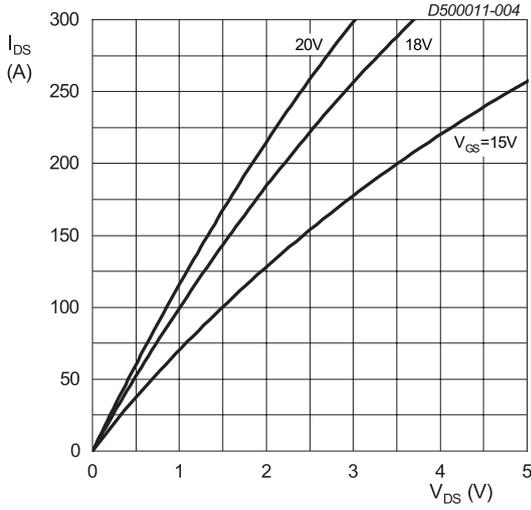
$T_j = -40\text{ °C}; t_p < 200\ \mu\text{s}$
