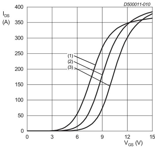
$V_{DS} = 20\text{ V}; t_p < 200\ \mu\text{s}$
