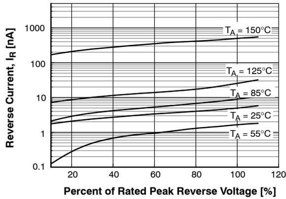
Figure 2. Typical Reverse Current Characteristic (Per Diode)
