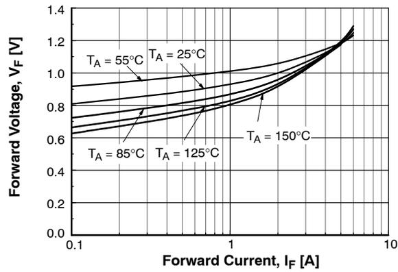
Figure 1. Forward Voltage vs. Forward Current (Per Diode)
