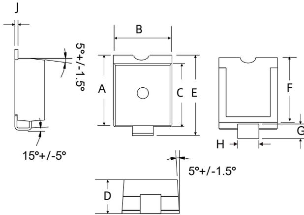
Note: Coplanarity of solder side is controlled within 0.10 mm
