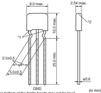
\*1 The bottom of the ferrite beads may not be level with each other.
