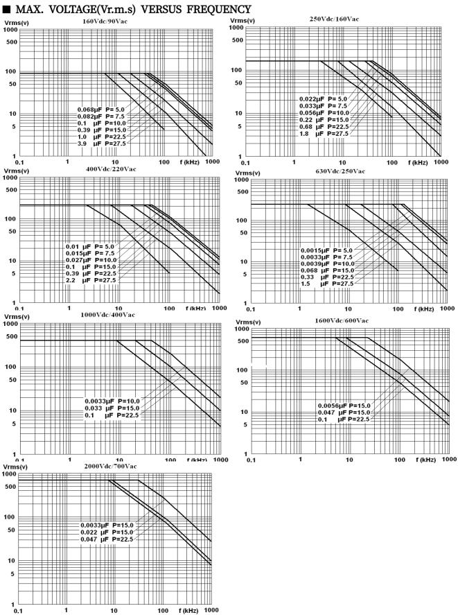
Note: sinusoidal wave-form, environment temperature  $\le$  85 °C ,internal temperature rise  $\triangle$  T=10 °C , p (pitch) in mm..
