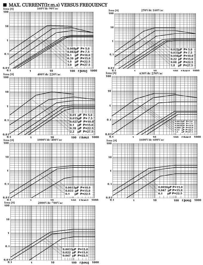
Note: sinusoidal wave-form, environment temperature  $\leq$  85 °C, internal temperature rise  $\triangle$  T=10 °C, p (pitch) in mm.
