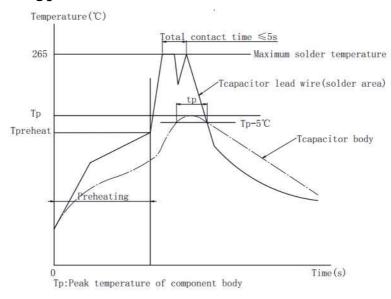
▲ Because overheating could damage the capacitor, we recommend paying attention to the maximum capacitor temperature and heating time, use temperature sensor to detect the maximum capacitor body temperature.
