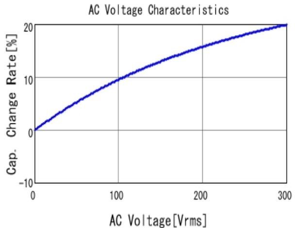
■ DE2B3KY101KN3AU02F C-AC Voltage capchange, DC0V, 20.0
