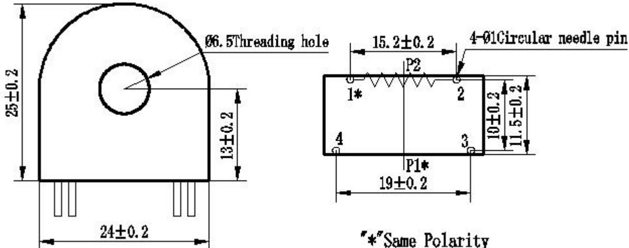
Remarks: Primary input: straight-through type (make the measured circuit be through the hole)
