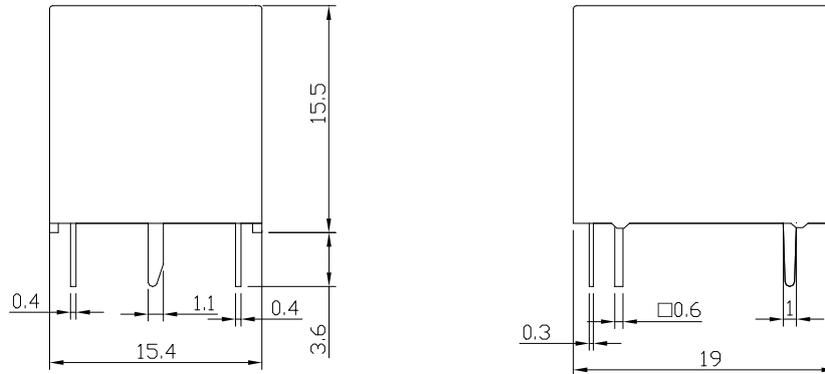
Dimension tolerance not shown in the dimension of installation hole installation holes are all  $\pm 0.2\text{mm}$ .
