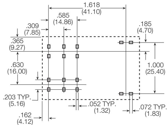
An alternate PC board layout utilizes .076 ± .003 (1.93 ± .076) diameter holes on the same center-to-center spacing shown above. Use of the rectangular holes is recommended for improved solderability.
