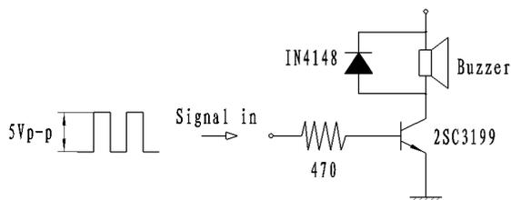
Resonant frequency, 1/2 duty cycle. Square wave.
