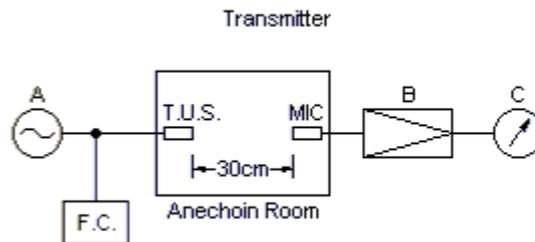
A: Oscillator B: Amplifier C: Voltmeter MIC: Microphone
