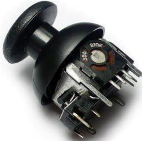
This is a joystick very similar to the 'analog' joysticks on PS2 (PlayStation 2) controllers. Directional movements are simply two potentiometers - one for each axis. Pots are ~10k each. This joystick also has a select button that is actuated when the joystick is pressed down.
