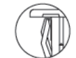
DETAIL VIEW VH1, VH3 & VH5 HOLE PLUGS (No wing serrations for ease of removal)
