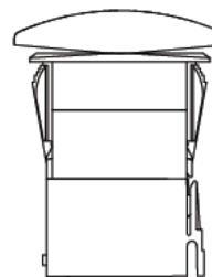
SWITCH SHOWN WITH VC1 CONNECTOR 10 TERMINAL
