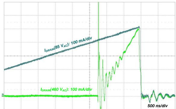
Figure 30.  $I_{LIMIT}$  Waveforms (85 V<sub>AC</sub> vs. 460 V<sub>AC</sub>)
