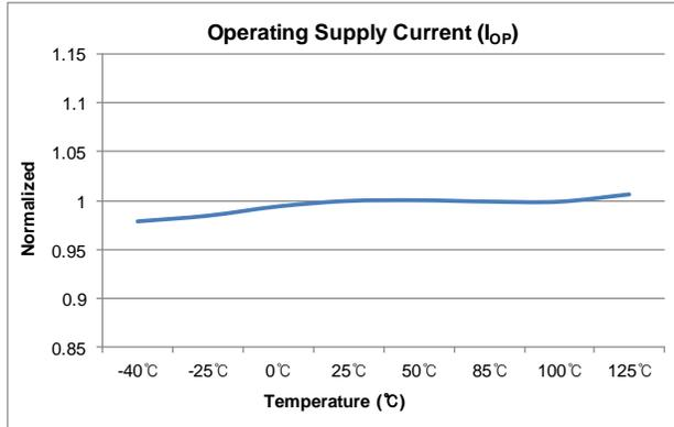
Figure 5. Operating Supply Current ( $I_{OP}$ ) vs.  $T_A$
