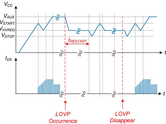
Figure 25. LOVP Waveforms
