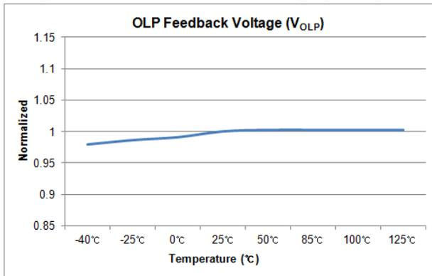
Figure 13. OLP Feedback Voltage ( $V_{OLP}$ ) vs.  $T_A$
