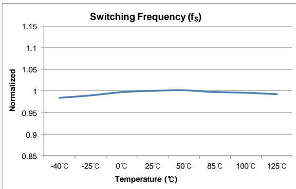
Figure 15. Switching Frequency ( $f_s$ ) vs.  $T_A$
