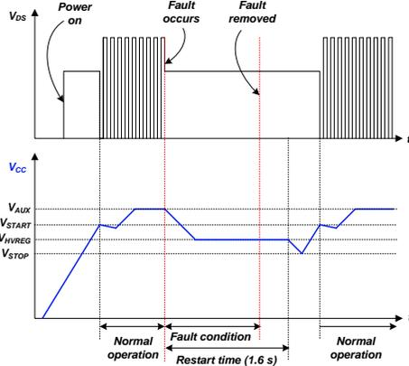
**Figure 19. Auto-Restart Protection Waveforms**
