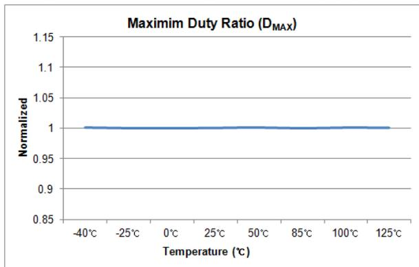
Figure 16. Maximum Duty Ratio ( $D_{MAX}$ ) vs.  $T_A$
