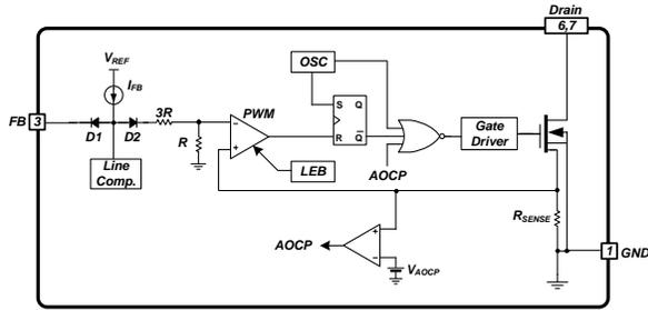
Figure 23. AOC Circuit
