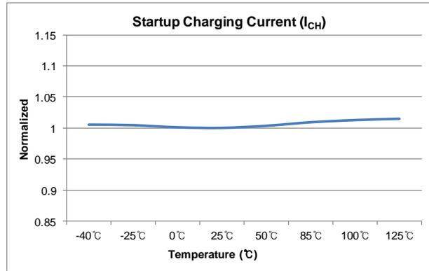
Figure 7. Startup Charging Current ( $I_{CH}$ ) vs.  $T_A$
