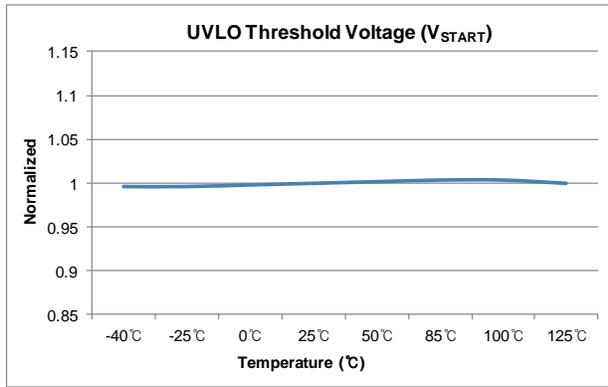
Figure 11. UVLO Threshold Voltage ( $V_{START}$ ) vs.  $T_A$
