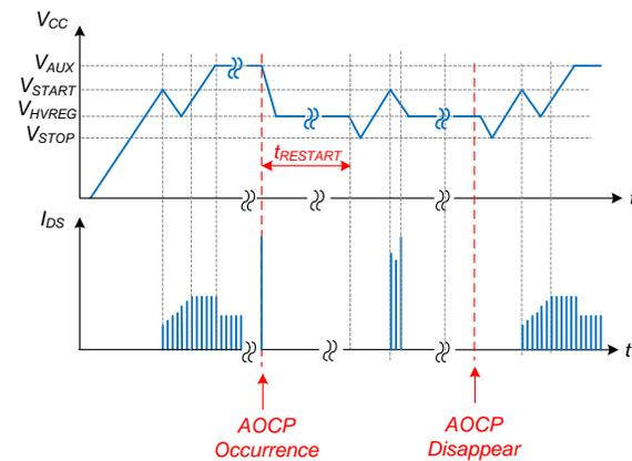
**Figure 22. AOCP Waveforms**
