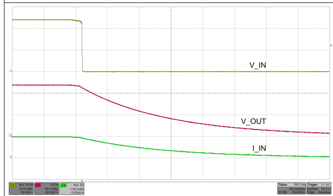
Figure 56. Start-Up With VIN—48-Ω Load
